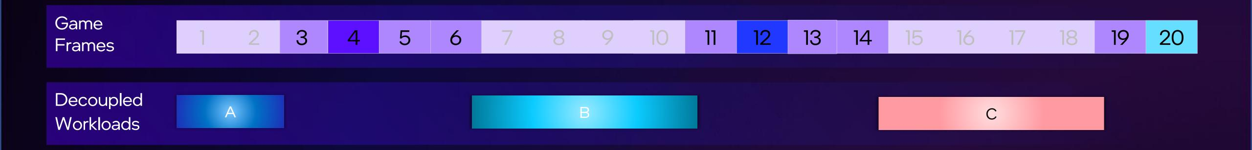
Frames  $3\rightarrow 6$  and  $11\rightarrow 14$  and  $19\rightarrow 20$  will execute more quickly due to no overlap with Decoupled Workloads.
